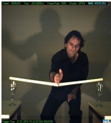
Fig. 2. Snapshot of a high speed video sequence: a wooden rod is hit by a fast moving hand at its center. While breaking, the ends move upward such that the supports are not damaged.
