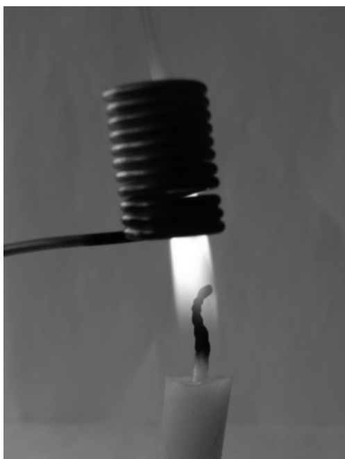
Putting out a candle and lighting it again by a metallic spiral
