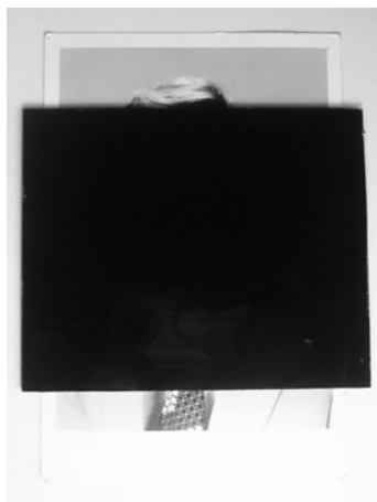
Fig. 1 Picture of a black-and-white photograph covered with a black filter taken in the visible light mode.
