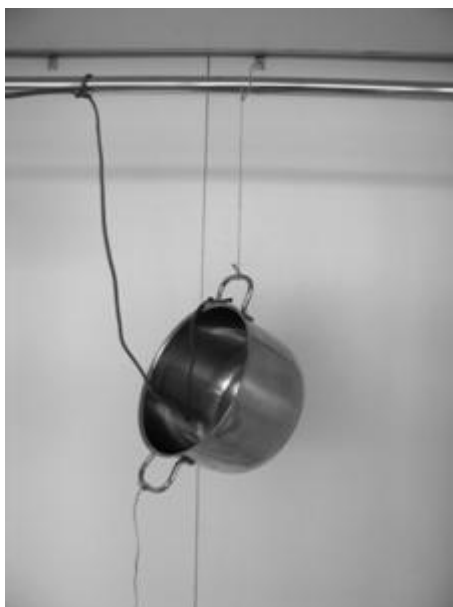
Fig.3: The pot prepared for the breaking of the string. The thicker string acts as a safety device to prevent the pot from striking the floor.
