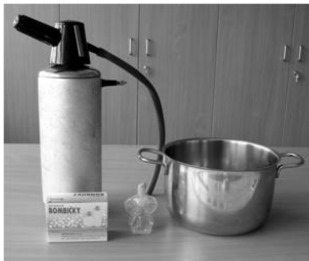
Fig. 4: Tools required for demonstrations of Archimedes' Law in \text{CO}_2
