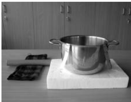
Fig. 1: The pot acting as an electroscope
