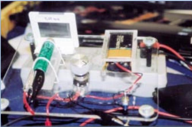
We can verify an order of magnitude for the speed of light by measuring the wavelength of red light from a laser pointer and the striking voltage of the laser diode.
