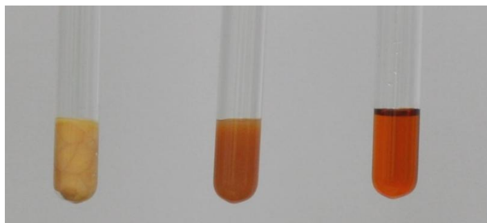
Figure 6. Liquid crystal MBBA in different phases: (a) Crystalline; (b) Liquid crystalline (nematic) and (c) Liquid. Liquid crystal MBBA has a melting point 20 °C and a clearing point 41 °C [13,14].
