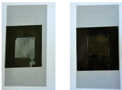
Figure 9. (a) A drop of liquid crystal MBBA (anisotropic) and (b) a drop of water (isotropic) between two polarizers with perpendicular polarizer axes [10]
