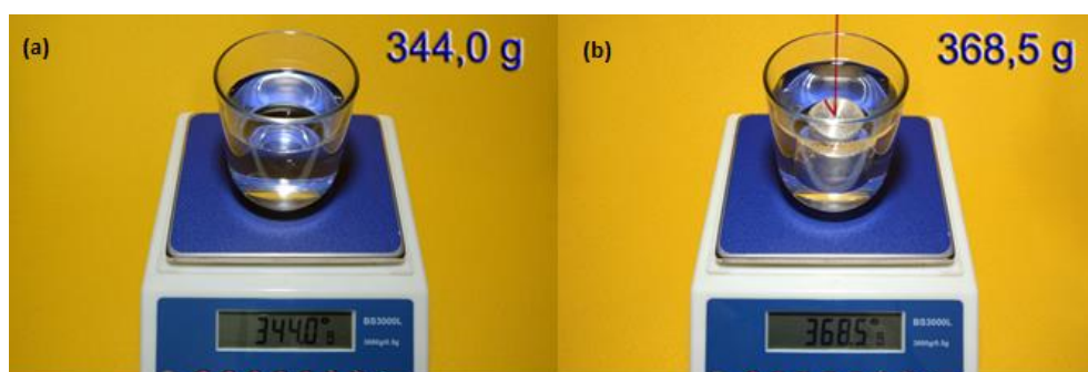
Fig. 5. (a) Mass of the beaker of water; (b) Mass of the beaker of water with cylindrical object inside
