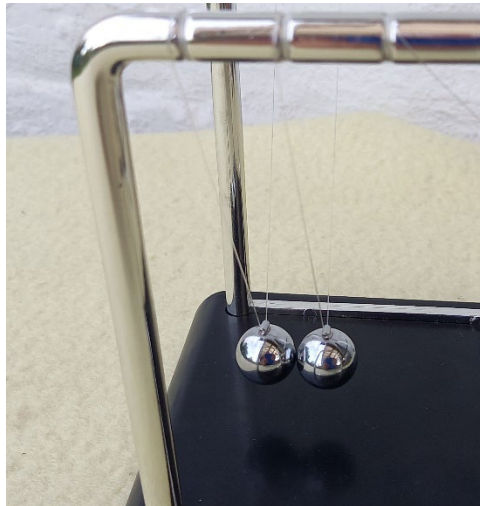
Fig. 1. A model of neutron-proton collision demonstrated on a Newton's cradle. The incoming ball stops and the other one flies away at almost the same speed.
