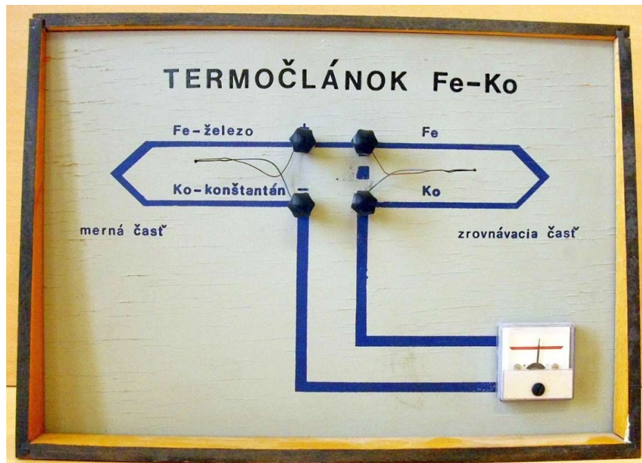
Fig. 4. a pair of thermocouples on a panel is a fitting example of permanent physics experiment. Always ready for action, no adjustments needed.
