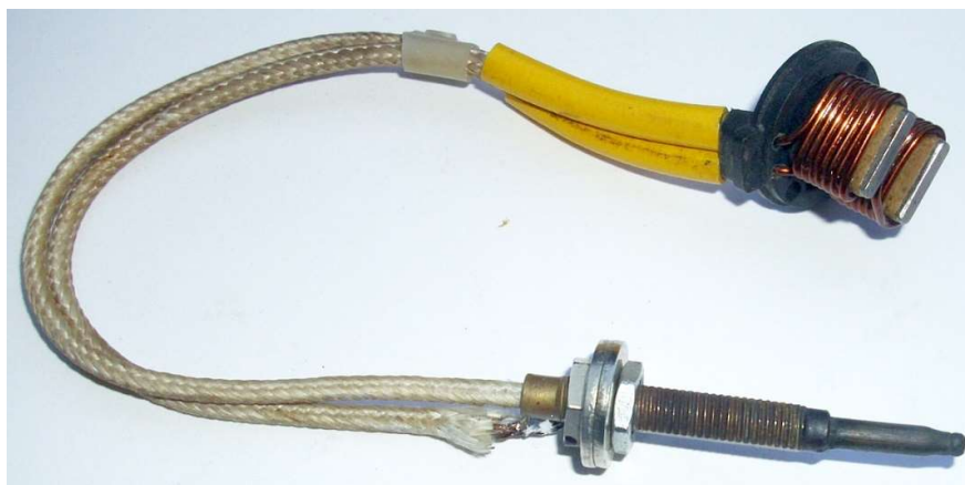
Fig. 6. Thermocouple in brass tube powers an electromagnet. For the electromagnet to properly function only voltage of approx. 10–20 mV is needed. This voltage ensures that the current flowing through the circuit is in the order of tenths of ampere.
