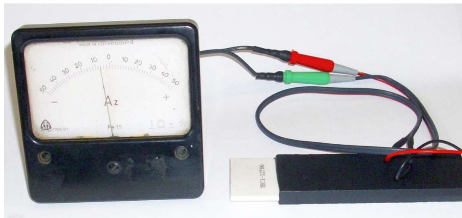
Fig. 8. Typical permanent experiment, Peltier connected to galvanometer. All that is required for maximum displacement is touch of a finger. Touching other side of the device causes current to change direction and consequently pointer displaces itself in the other direction as well. It is obviously possible to touch the device with a cold object e.g., a piece of ice, which causes current to flow in opposite direction.
