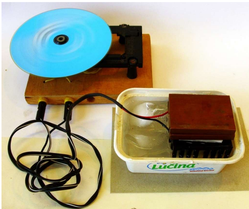
Fig. 10. Peltier device mounted on top of computer passive cooler. Cooler is being cooled by ice cold water in which it is submerged. There are two copper prisms on top, that were originally heated in hot water to temperature of approx. 50 °C. In this arrangement Peltier device yield approx. 1,3 V and current 150 mA.
