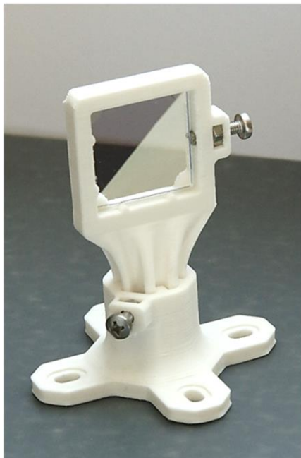
Figure 12. Completed beam splitter module
