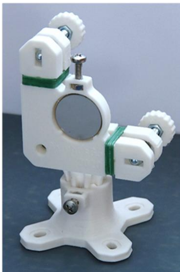
Figure 16. Completely assembled module with a mirror
