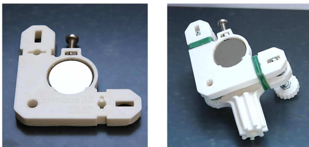
Figure 15. Mirror holder on the left, assembled upper part on the right
