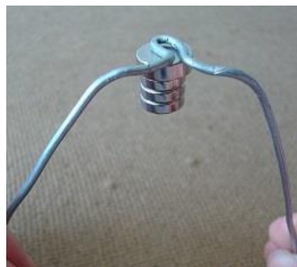
Figure 5 – Metal structure for insertion of neodymium magnets into the coil cavity
