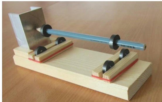
Fig. 1 – Magnets' repulsion used to make a pencil levitate (adapted from [3]).
