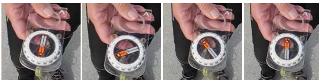
Fig. 7: When lowering the north end of the needle towards the ground the needle rotates 180°.
