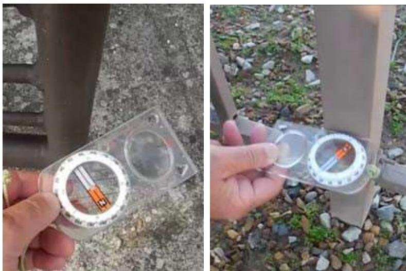
Fig. 6: On the left – attraction of the compass needle to a vertical iron bar on the Northern Hemisphere; on the right – on the Southern Hemisphere.
