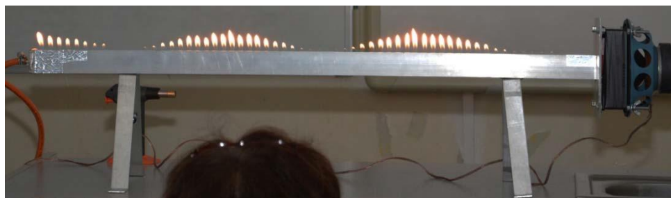
Fig. 3: Example of the shape of the flames
