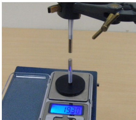
Picture 5: Measuring of the force between two magnets ( l = 25 mm, R = 2.5 mm)
