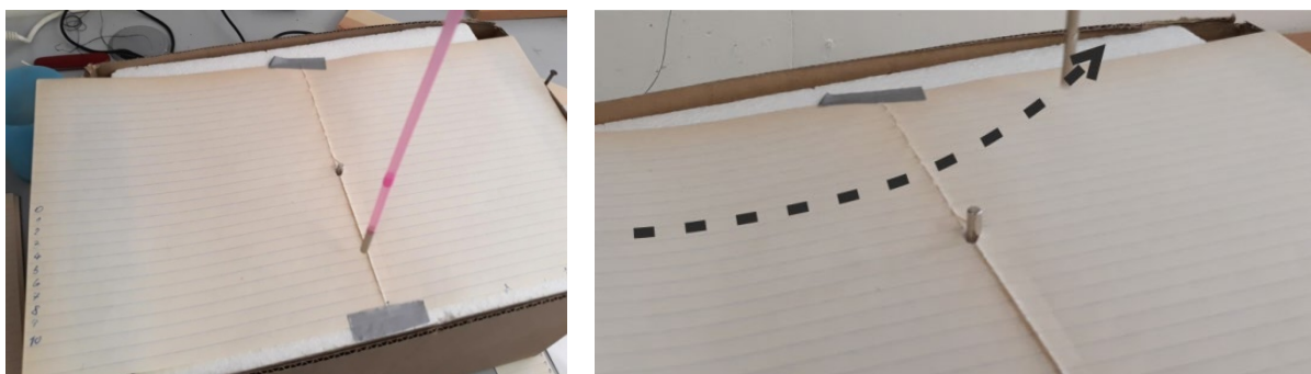
Picture 1: Model of Rutherford’s experiment, in which the repulsion acts between the poles of the magnets
