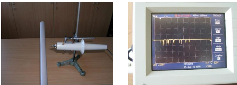
Fig. 3 Discharge of charge from a charged PVC rod to the tip of the probe
