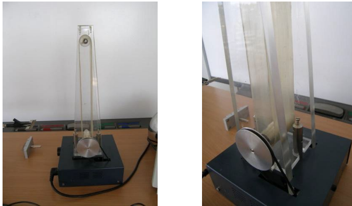
Fig. 6 School Van de Graaff generator without the collecting brushes
