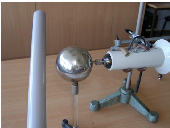
Fig. 6. Discharge of the rod into a metal ball attached to the probe tip
