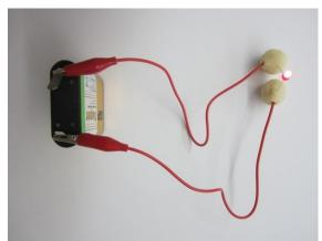
2. Serial wiring of 2 LEDs
