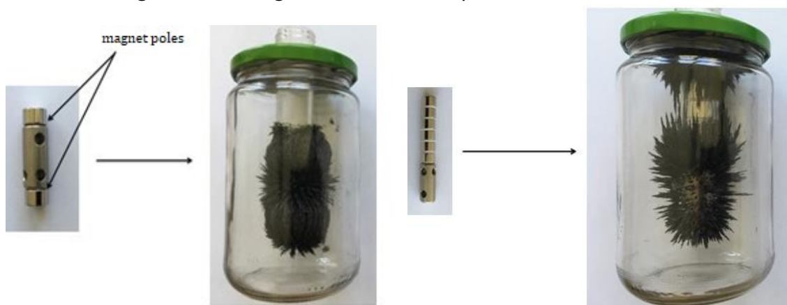
Fig. 5. On the left, two magnets with corresponding poles facing each other and an iron cylinder between them. On the right, an iron cylinder attached to a cylindrical magnet.
