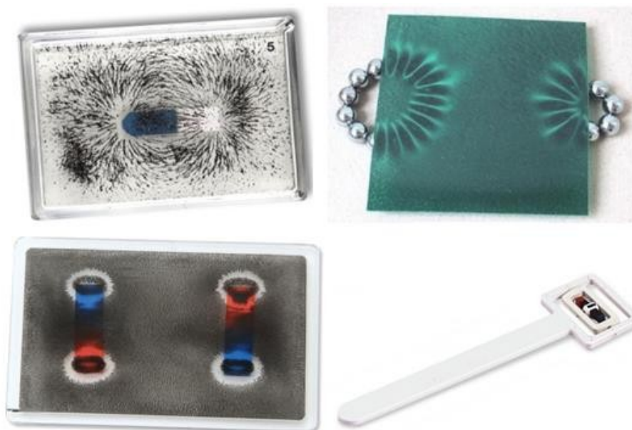
Fig. 1. Magnetic field investigation using: iron filings, sensor foils, detection plates, magnetic field sensors.
