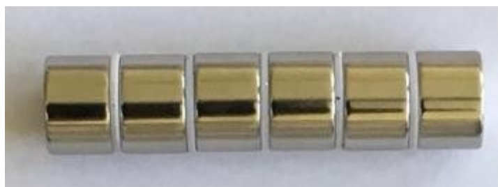
Fig. 4. Cylindrical magnet composed of 6 neodymium magnets (one magnet has a diameter of 15 mm, height of 10 mm)
