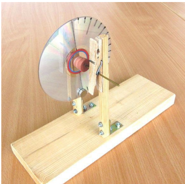
Fig. 1. Simple pendulum design with large oscillations
