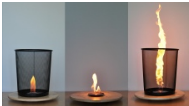
Picture 10: Fire in the non-rotating basket. Fire on the rotating tray. Fire on the rotating tray in the basket.
