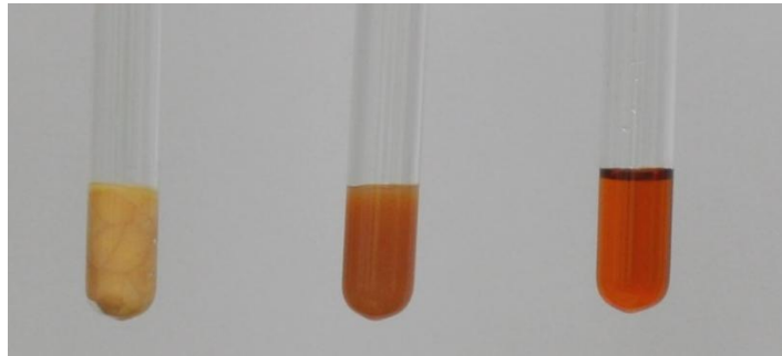
Figure 6. Liquid crystal MBBA in different phases: (a) Crystalline; (b) Liquid crystalline (nematic) and (c) Liquid. Liquid crystal MBBA has a melting point 20\text{ }^{\circ}\text{C} and a clearing point 41\text{ }^{\circ}\text{C} [13,14].
