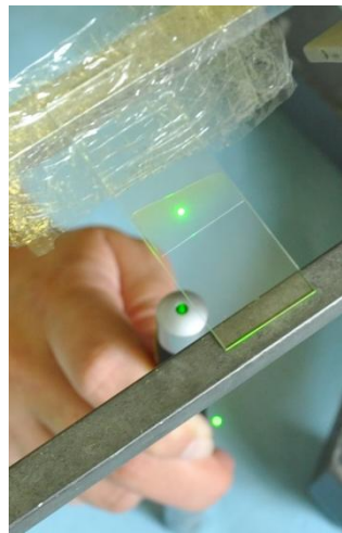
Figure 11: Experimental setup for demonstrating the double refraction
