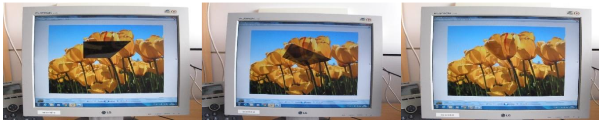
Figure 8. Different position of the polarizer on the screen. One can conclude that light from the screen is polarized.
