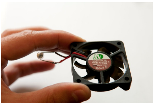
2: Fan as a source of electrical energy
