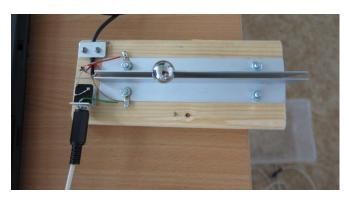
sible solution are shown in the photo. Metal ball lies on two small "rails" which, in our case, are made of two aluminium L-shaped sections screwed to a wooden board. Distance between the sections is about 4 mm. Rails are connected in parallel to the microphone which is connected to a computer's microphone input. As long as the ball is lying on
