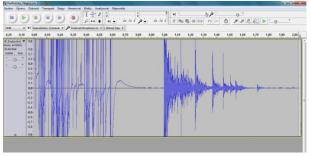
point where the ball leaves the rails still can be well located. (Let us add two technical notes: 1. Decreasing of the signal and its overshoot after the last impulse is probably given by capacitors in the computer's microphone input. 2. The ball has to have a certain minimum velocity on the rails so that it did not flip over the end edge slowly; calculation will show that for a small ball the velocity of about 40 cm/s is enough.)
