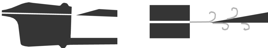
Picture 1 – On the left: section view of a recorder's fipple. On the right: blowing air through the channel to the sharp edge and forming vortices.
