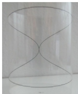
Fig. 7 Lissajous curve for frequency ratio 2:1
