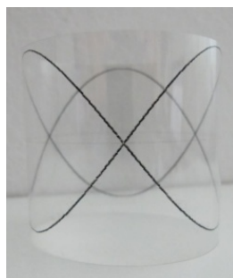
Fig. 8 Lissajous curve for frequency ratio 2:3
