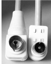
Fig. 5 Close-up of the connectors of the transmitter antenna (left) and the receiver antenna (right)
