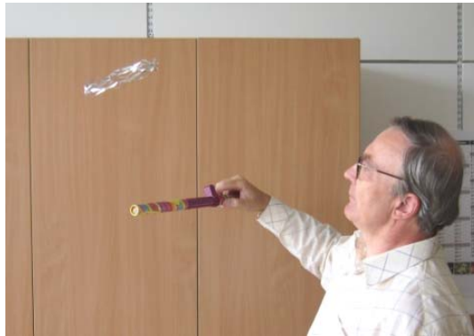
Fig. 2 The charged end of the wand repels a foil ring that was previously charged with the wand
