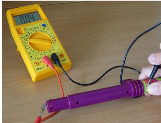
Fig. 6 Measuring the current provided by the magic wand. (The photograph does not show the decimal point in front of the last digit; the readout is 0.4\ \mu\text{A} ).
