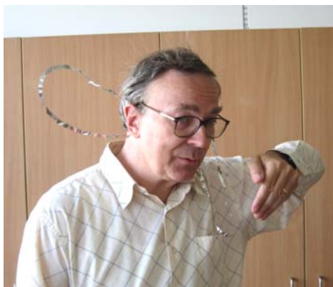
Fig. 9 A foil strip in a “hollow” between the head and the hand is hanging down because the electric field is (approximately) zero there. (The strip on the other side is repelled from the head indicating that the man is really charged.)
