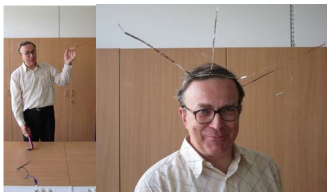
Fig. 8 Magic wand charges a man – the result is demonstrated by hair or foil strips
