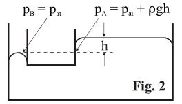
If the liquid surface between the vessel wall and the floating object forms convex meniscus then under the surface curved in such a way the pressure is higher than the atmospheric one:
