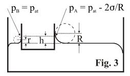
If you move the object towards the vessel wall then similarly as in previous cases the liquid surface will be curved more but in this case at one wall a bigger curvature of concave meniscus will be formed and at the other wall a bigger curvature of convex meniscus will appear. The level of liquid will not change because the surface between meniscuses does not form a curve  $(2\sigma/r = 0)$ .
