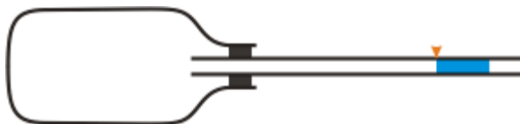
Fig. 1: If the tube is horizontally oriented, inside the bottle is the same pressure as in the surrounding atmosphere
