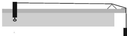
It is possible to support the string by a “bridge” – a piece of L-shaped metal profile that changes the length of the vibrating string. By changing its position you can show the dependence of tone pitch on string length. Use a similar piece to protect the edge of the table from notches made by the string.
