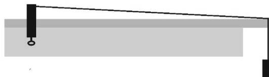
If you pluck the string you will find that its sound is very quiet. Put the neodymium magnet into the core of the coil and connect the coil to the amplifier. Now pluck the string again and approach the vibrating string with the coil so that the magnet is about 5 mm away from the string. The speaker should sound with a clear guitar tone.
