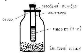
Make a hole the size of a test tube in the screw lid. Put magnets into the test tubes, plug them and twist a rubber band around the top. Pour the filings into the jar and close it by the prepared lid. Then push the test tubes into the hole in the lid, shake the jar, and observe the formed chains of filings.
