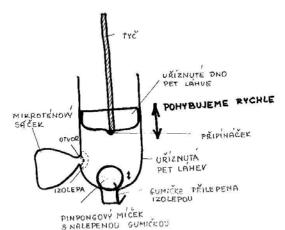
If we move the piston up, low pressure appears inside the bottle, so the air from outside is sucked through the bottle mouth together with dust and rubbish. After pushing the piston the air pressure rises andthe ball is pressed down to the bottle mouth. The only place where the air can leave now is the hole on the side of the bottle where the bag is glued.
