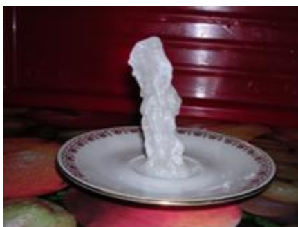
Fig. 5 Column created by pouring of supercooled solution on some crystals of sodium acetate
