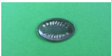
Fig. 4 The tinny disc that starts crystallization in the heat pack
