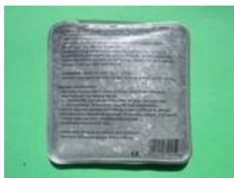
Fig. 3 Cold heat pack with some unmelted crystals of sodium acetate
