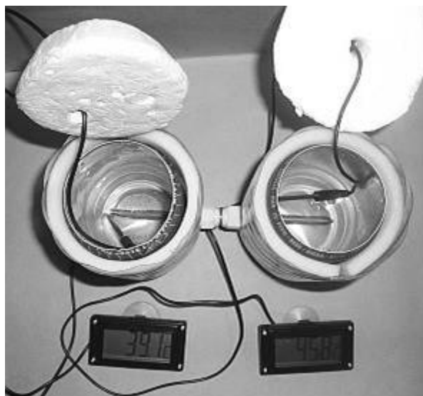
Fig. 5: Calorimeters made of beer cans connected with a heat pipe
