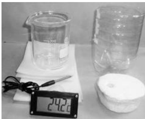
Fig. 4: Parts for manufacturing of a calorimeter. A digital thermometer is not necessary but very useful. It is mechanically durable and sufficiently sensitive.
