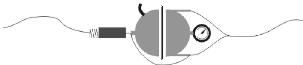
The advantage of this device is that its demonstration involves all the students in the class. We pump the air out of the hemispheres and close the inlet. Then students come one by one to the ropes and try to pull the hemispheres apart. We can read both the pressure inside the hemispheres from the vacuum gauge and the pulling force that is needed to pull the hemispheres apart. Then we can compare these values to the theoretical calculation of the force
