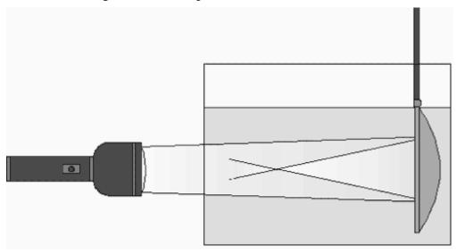
3. A horizontal laser beam travels through a bent piece of Perspex that is in an aquarium (see the figure below). Total internal reflection takes place (no part of the beam leaves the Perspex at the point of incidence).
