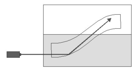
4. The beam hits the top surface of the Perspex with much smaller angle of incidence than in case 3.
