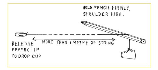
Take about 1.5 metre of string. Tie one end to the handle of a (cheap) teacup and the other to an ordinary paperclip. Hold a pencil horizontally in one hand – at shoulder height. Hold the paperclip in the other hand and draw the string across the pencil until the cup is hanging about 1.5 metres above the floor.
