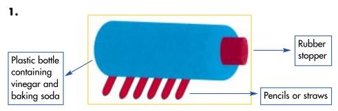
Place a teaspoon full of baking soda and 10mls of vinegar inside the plastic bottle. Quickly replace the rubber stopper. After a few seconds the build up of pressure from the carbon dioxide causes the stopper to fly off in one direction while the bottle shoots back in the opposite direction. By placing the bottle on rollers such as pencils the effect is enhanced.
