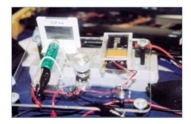
We can verify an order of magnitude for the speed of light by measuring the wavelength of red light from a laser pointer and the striking voltage of the laserdiode.
