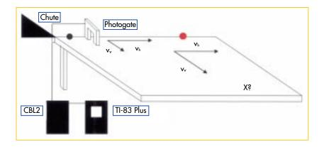
(Note: The chute must direct the ball-bearing straight across the top of the inclined plane, i.e. to ensure it possesses no vertical velocity component at the start of its motion on the plane.)
