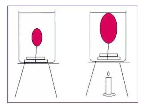
The balloon on the left is submerged in a beaker of ice-cold water. When the water is boiled, the gas is heated and it expands.
