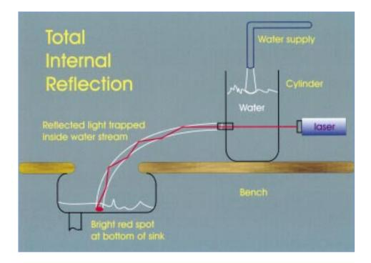
Drink a bottle of mineral water! Cut a small circular hole in the side of the bottle. It helps to fit a centimetre or so of plastic tubing or drinking straw (not too narrow) in the hole. Stand the bottle beside a sink and under a tap so that a steady stream of water pours into the sink. Now shine a laser beam through the bottle and out into the water stream. Note how the water acts as a light guide.
