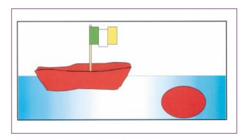
The boat and ball both made from Plasticine, each have equal masses (weights), but because of it's shape the boat floats, while the ball sinks.
