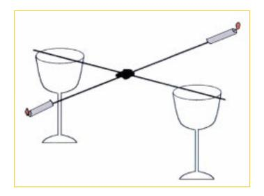
Use kebab sticks and blue tack to assemble this demonstration. Candles will oscillate when lit demonstrating balance.
