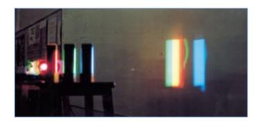
Make a transparency with **RED**, **GREEN** and **BLUE** filters, side by side. For a 35mm slide you need only three pieces of filter about 15mm x 30mm. These may be slightly overlapped and fitted into, or taped onto a 35mm slide mount. For the OHP version take a sheet of card at least 300mm x 300mm and cut three similar holes. Tape sheets of red, green and blue filter over the three holes. Place your three coloured windows on the stage of the OHP.
